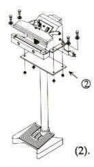
(3). Attach puller rod to puller (localed under base) and then attach to foot pedal.
